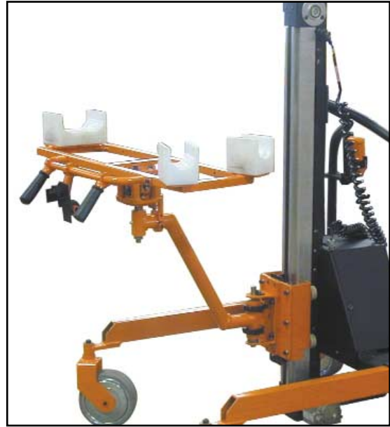
End effector for positioning an exhaust system onto a vehicle.
