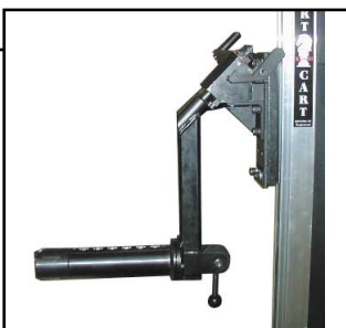
Detail of the roll handling end effector.
